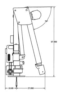
**HOIST WINCH:** The hoist winch uses a planetary gear drive for most efficient operation. The winch is powered by a permanent magnet electric motor. The single line capacity of the winch is 1200 Lbs. An integral mechanical brake is included with the winch.
