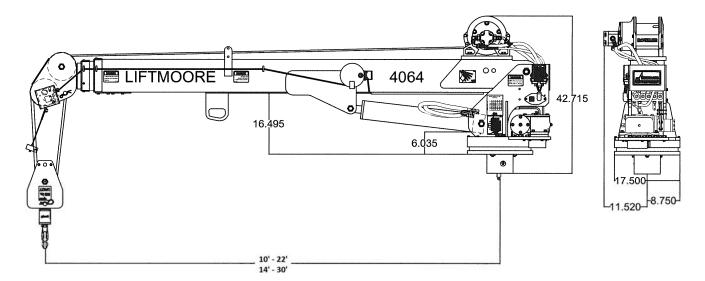
**CAPACITY:** Moment rating of 40,000 ft.-lbs. with lift capacities as follows.
